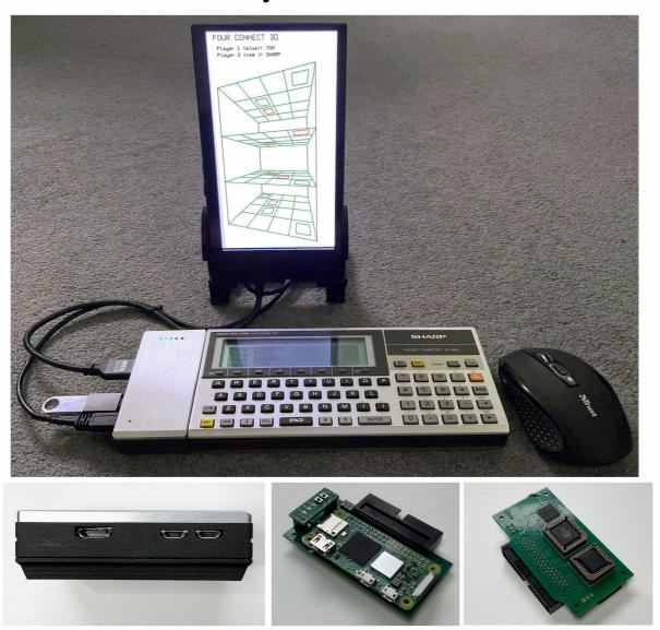
This module is the modern equivalent of the CE-1600P DIN A4 plotter and the CE-1600F disk drive. It fully integrates with the PC-1600 OS.
