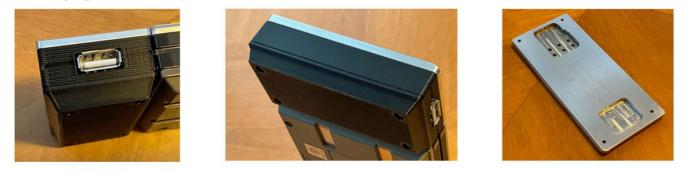
The module fully integrates with the PC-1600 OS and presents the memory stick as a device S3. So read and write access is as easy and natural as with a RAM-disk S2. Supported standard commands: FILES, [B]SAVE, [B]LOAD, COPY, KILL, NAME, OPEN, PRINT#, INPUT#, CLOSE Plus two extra commands from the modules ROM extension: CDIR: Change directory on the memory stick (UNIX-style) LDIR: List subdirectories of current directory
